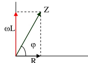
$$\text{tag} \varphi = \frac{L * 2\pi * f}{R} = \frac{1,2 * 2 * 3,14 * 50}{166,3} = 2,27 \Rightarrow \varphi = 66,2^\circ$$
